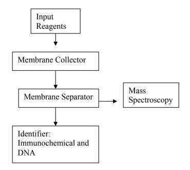
Figure 1. Nanoporous membrane identification system for ultrafiltration.
