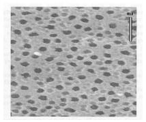
Figure 3. SEM of the pore distribution of Anodisc alumina membrane
