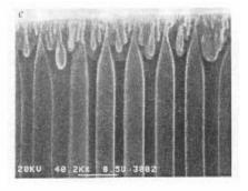
Figure 2. Cross sectional SEM image of Anodisc alumina membrane
