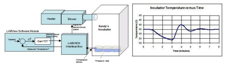
A bioengineering graduate student built a simple incubator to support her cell growth experiment. Her experiment requires repeatedly opening the door to sample the cells. When the door is closed the performance of the system was less than optimal as shown by the overshoot in temperature at 4 seconds.
